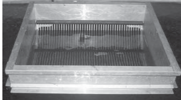
Figure 24. The use of a grader box should result in a more uniform harvest.
